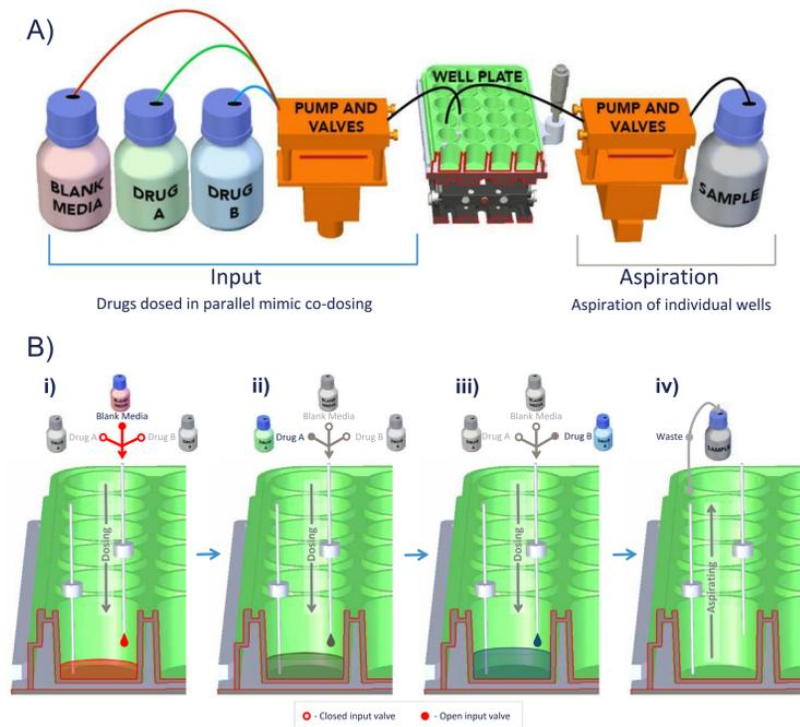
**Figure 3 – Microfluidic addition and removal device for PK modelling *in vitro***
