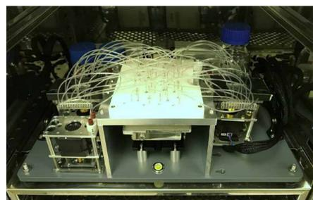
**Figure 1 - Microfluidic addition and removal device**
